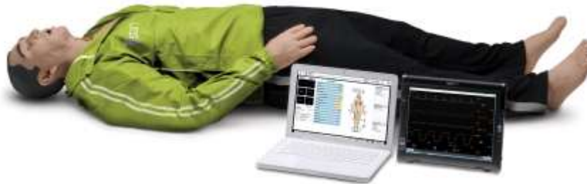
Figure 4-3: iStan is a wireless patient simulator with fully articulated movement and advanced features
